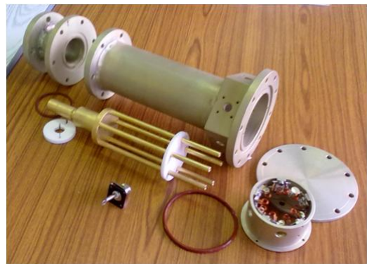
Figure 3 Photograph showing different parts of the five way in- phase equal power divider/combiner
