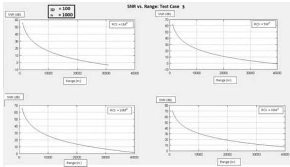
Fig. 6. Results: Test Case - 3 ((SNR vs Range at ID = 100 and n = 1000)
