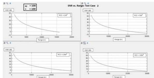
Fig. 5. Results: Test Case - 2, ((SNR vs Range at ID = 100 and n = 100)
