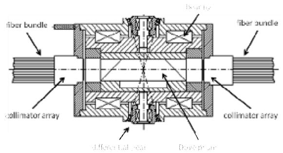
Figure 4 Fiber-optic multichannel module, longitudinal section
