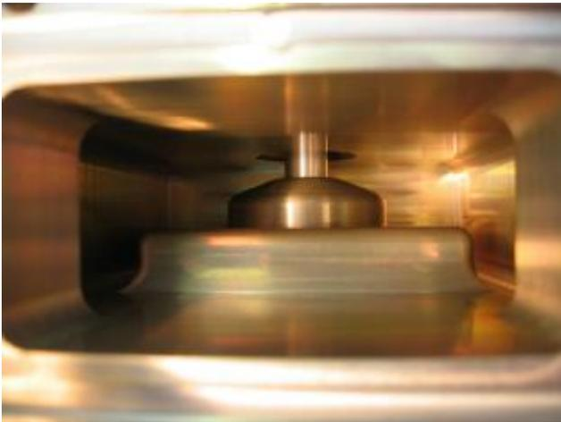
Figure 3 Details of door-knob type transition exhibiting the hollow center conductor
