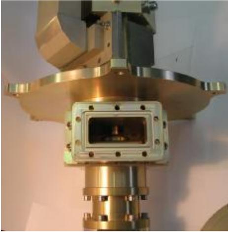
Figure 2 RF waveguide channel for high power operation at S-band
