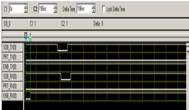
3. Figure : Delay between the enable control at POST MASTER and POST MAN
