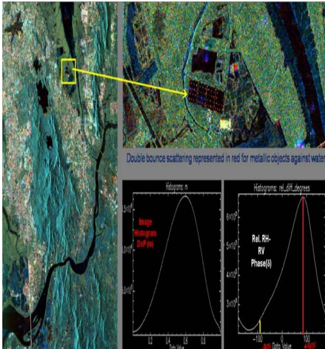
Figure: 1 RGB image (Mumbai area) generated with m- δ decomposition depicting Surface, volume and double bounce scatterings along with distribution of ‘m’ and relative phase between RH and RV.
