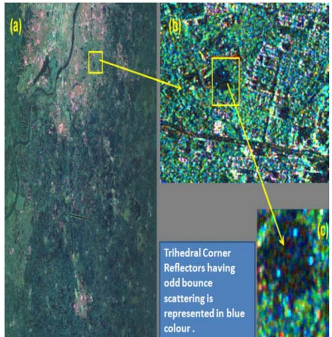
Figure: 2 (a) RGB image (Ahmedabad) generated with m- δ decomposition (b) Trihedral corner reflectors deployed at SAC campus (c) depicting odd bounce scattering shown in blue colour
