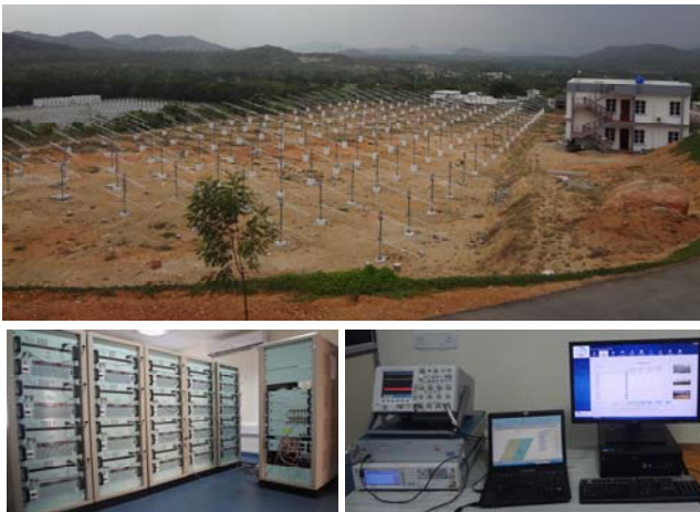
Figure-2: Photographs of the antenna array and the instrumentation building (top panel), transmit-receive system (bottom left) and radar controller (bottom right).
