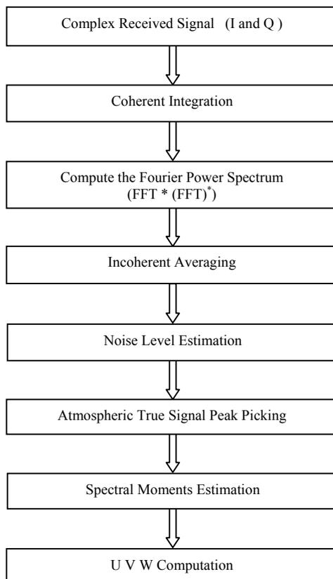
Figure 1. Classical signal Processing steps for wind velocity measurement
