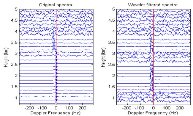
Fig. 5. Power spectra for all range gates (original and filtered) for east beam
