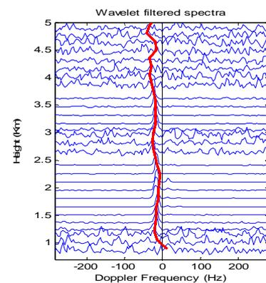
Fig. 6. Power spectra for all range gates with mean Doppler (red colour)
