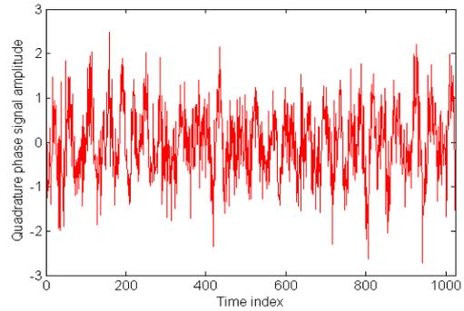
Fig. 3(c). Filtered 9<sup>th</sup> range gate quadrature phase signal
