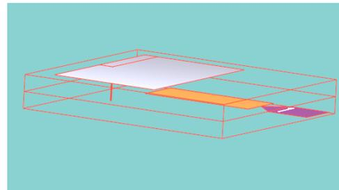
Fig 4. Schematic of Proximity coupled patch with DC short
