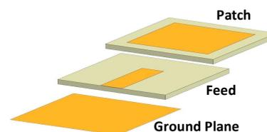
Fig 1: Schematic of Proximity Coupled Antenna
