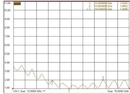
Fig 8. VSWR result of 4x4 Array Antenna
