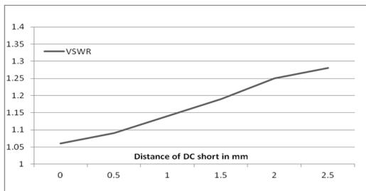
Fig 6. VSWR dependence on deviation of DC short from the center
