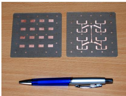
Fig 7. Hardware of 4x4 Array Antenna and Feed Network
