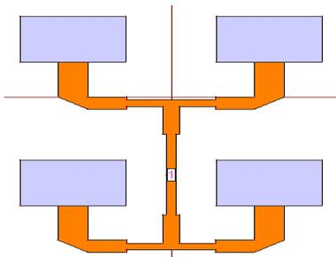
Fig 2: 2x2 Array scheme with feed network
