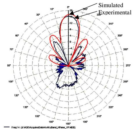
Fig 9. Comparison of Simulation & Experimental Patterns of 4x4 Array
