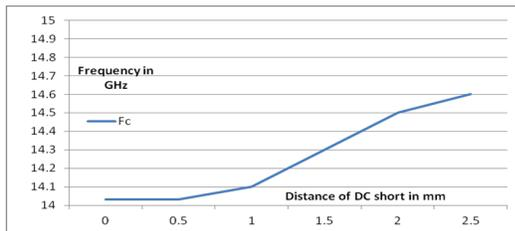
Fig 5. Resonating frequency changes on deviation of DC short from the center
