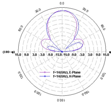
Fig 3(b): Radiation pattern in E & H planes for 2x2 array
