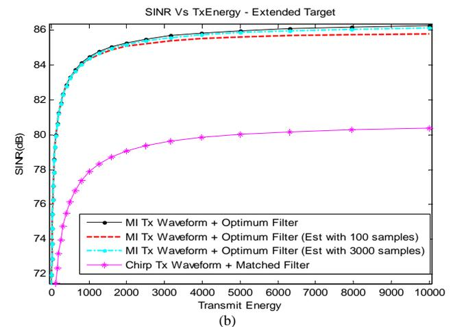
Figure 4. SINR Vs. TxEnergy with (a)100 samples and 3000 samples for estimation. Color coding of the plots is: MI with optimal Rx (black), MI with optimal Rx with estimation (red), Chirp with Matched filter (conventional) (magenta)
