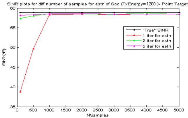
Figure 5. SINR plots for different number of samples for estimation (TxEnergy=1200). Color coding of the plots: Desired (black), 1 iteration (red), 2 iterations (green), 5 iterations (magenta)
