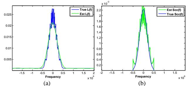
Figure 2. (a) True  $L(f)$  (blue) and  $\hat{L}_{lfm}(f)$  (green) (b) True  $S_{cc}(f)$  (blue) and  $\hat{S}_{cc}(f)$  (green) for 9000 samples and 2 learning cycle iterations
