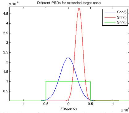
Figure 3. PSDs of extended target (red), clutter (blue) and noise (green)
