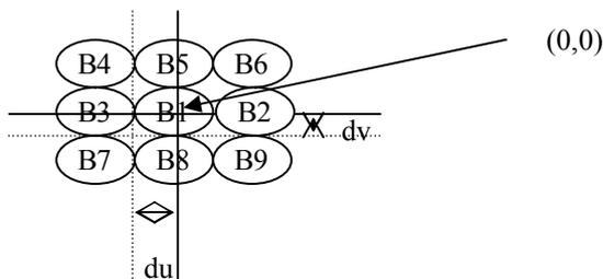
Figure 2. Beam offsets for 3 x 3 cluster of beams.
