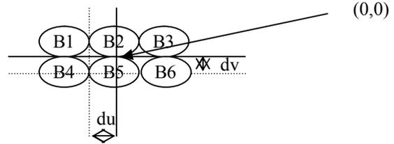
Figure 3. Beam offsets for 2 x 3 cluster of beams.
