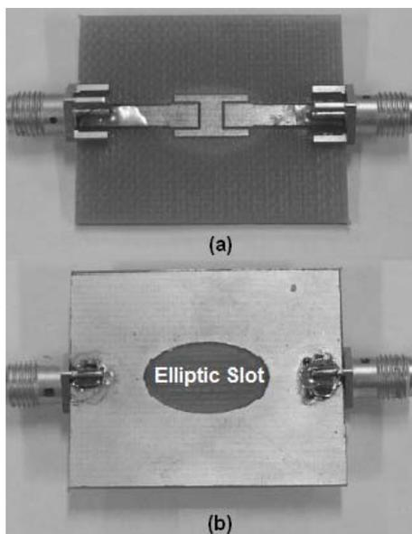
Fig. 6. Photograph of the UWB filter
