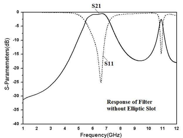
Fig. 5. Simulated results of filter without Elliptic shaped Slot
