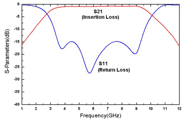
Fig. 4. Simulated results of proposed UWB Filter
