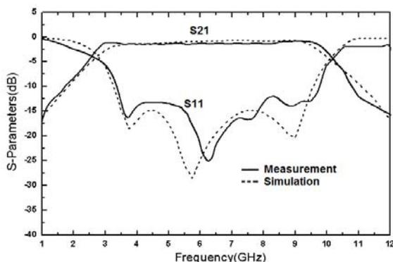
Fig. 7. Measured results of UWB filter
