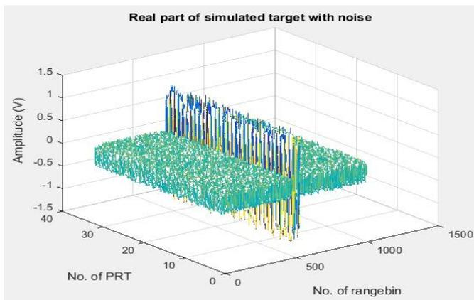
Fig. 5 Real part of simulated +12 dB Fr/2 simulated target data
