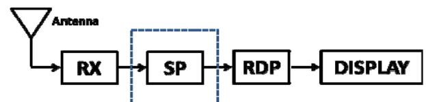
Fig. 1. Block diagram of radar receiving chain
