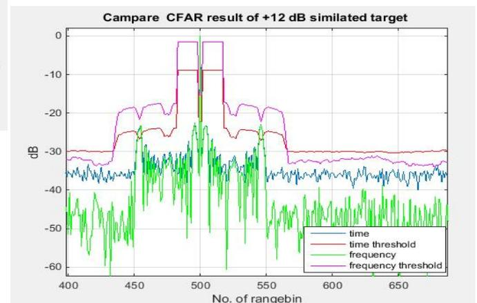
Fig.7 Compare CFAR result of +12 dB Fr/2 simulated target
