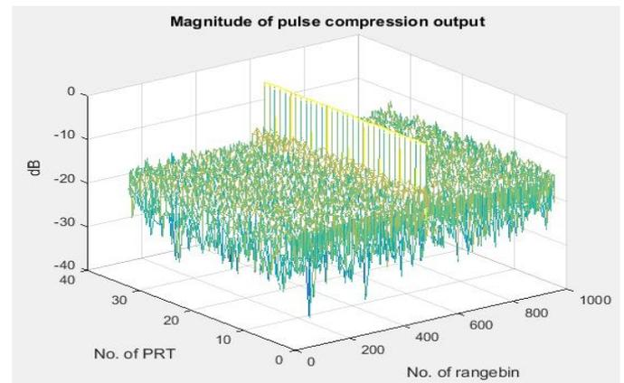
Fig.6 Pulse compression of +12 dB Fr/2 simulated target
