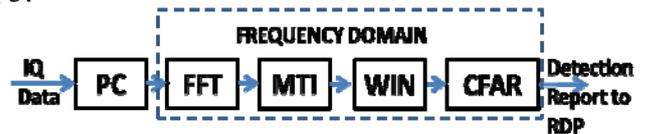
Fig. 3 Frequency domain radar signal processing chain
