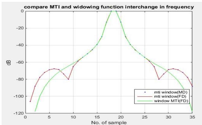
Fig.9 Compare MTI and window function interchange in frequency domain
