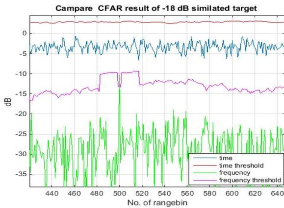
Fig.8 Compare CFAR result of -18 dB Fr/8 Doppler simulated target
