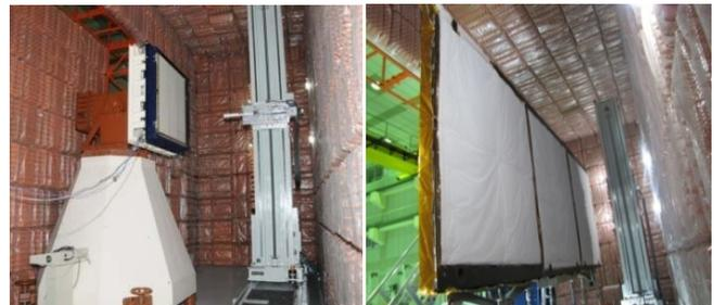
Fig.-3: RISAT-1 antenna test facility (Pulsed PNF) equipped with 3D scanning system. Left side image shows single antenna tile (24 TR elements) under test, whereas, right side image shows full antenna (288 TR elements) being scanned in Pulsed PNF
