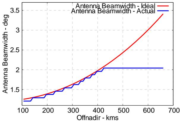
Fig.-2: In order to keep illumination swath constant across range swath, RISAT-1 Antenna beamwidth is being programically controlled w.r.t pointing by controlling antenna illumination along cross track. Figure shows variable beamwidth tracking required ideal beamwidth of antenna upto 420km swath, beyond that swath is controlled by return echo time.
