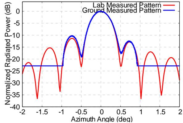
Fig-7: Comparison of measured Azimuth Antenna Pattern during testing in Lab and after launch ground measurement with a customized measurement setup. Results show a reasonable match upto first sidelobe.
