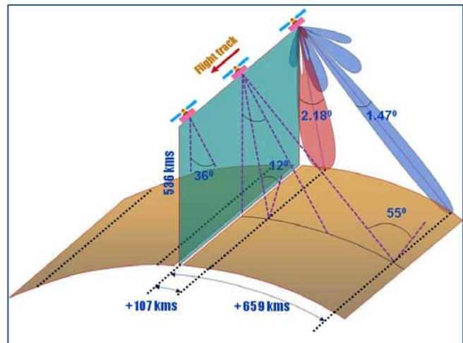
Fig.-1: RISAT-1 Antenna Beam Pointing showing Near and Far beams with variable beamwidth of 2.18 to 1.47 Range swath coverage from 107km to 659km is covered in 61 antenna beams with 10km step at spacecraft roll angle of 36° and nominal flight altitude of 536km.
