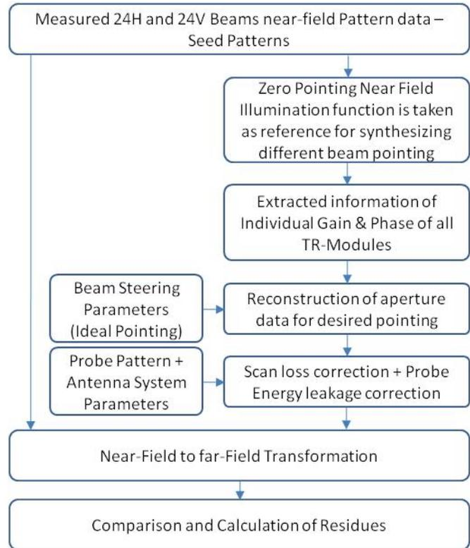
Fig-5: Antenna pattern synthesis flow in which Zero-pointing illumination function is taken as reference/seed pattern to synthesize all patterns using Beam-Steering parameters and probe pattern to compensate for scan-loss.
