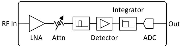
Fig-6: Block diagram of RISAT-1 antenna pattern measurement setup. Variable attenuator is used to bring down hardware dynamic range requirements due to orbital range variation in different satellite passes and beam pointing.
