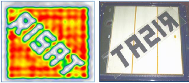
Fig-4: RISAT-1 active array antenna single tile carrying 24 TR elements showing absorber mask on the left side image and resolved near-field hologram for the same on right side image.
