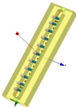
Figure 5 Simulated filter models with top cover plate removed
