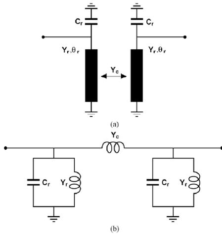
Figure 2 Second-order combline filter (a) topology (b) equivalent-circuit network
