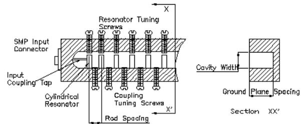
Figure 3 Mechanical structure of the Combline band pass Filter
