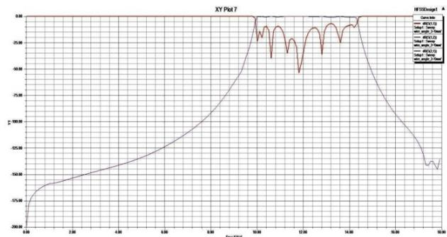
Figure 6 Simulated filter response
