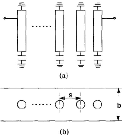
Figure1 Comblin filter with (a) plane view (b) cross section view
