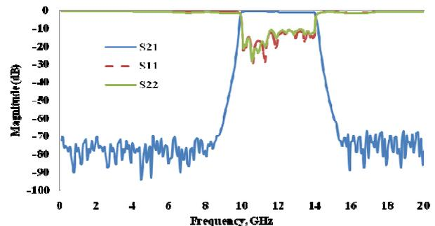
Figure 7 Measured filter response
