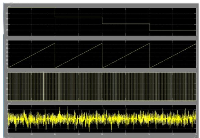
Figure 5 Total model output. a – Enable instantiated outputs, b – Count intervals, c – Generated enable signals, d – Sum output
