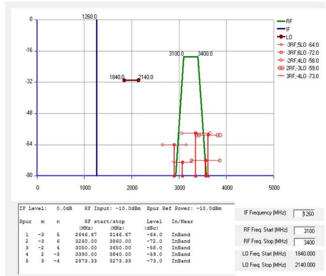
Fig. 4: Spurious analysis for S-Band receiver for mixing stage
