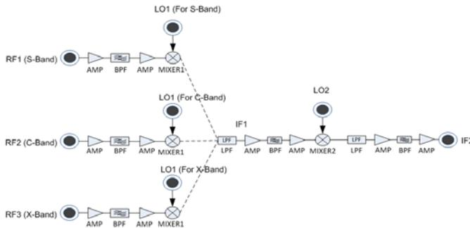
Fig. 3: Two stage down-conversion of proposed architecture
