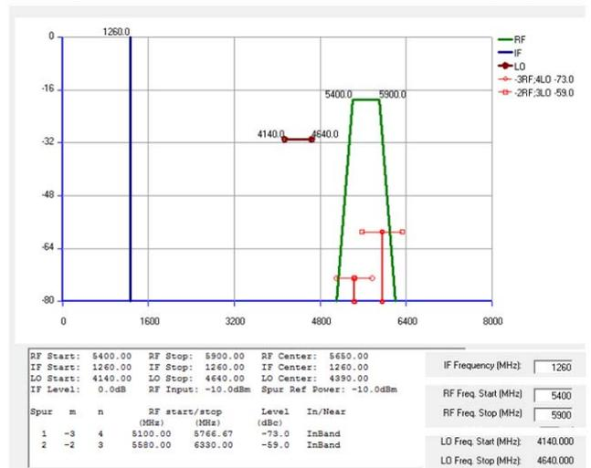
Fig. 5: Spurious analysis for C-Band receiver for first mixing stage
