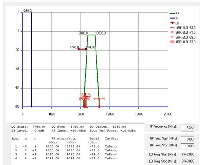
Fig. 6: Spurious analysis for X-Band receiver for first mixing stage
