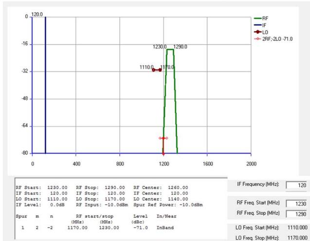
Fig. 7: Spurious Analysis for second mixing stage
