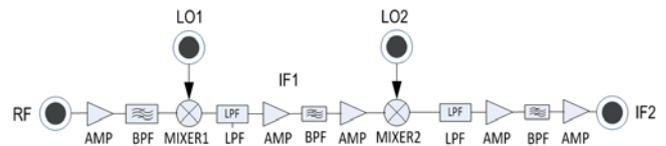
Fig. 1: Super heterodyne receiver architecture
