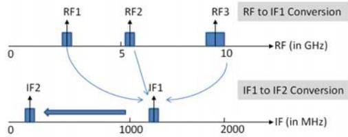
Fig. 2: Two stage down-conversion of proposed architecture
