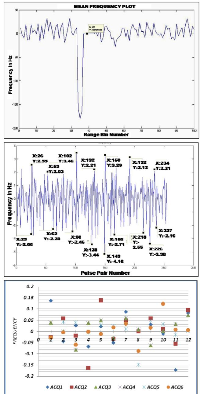
Figure – 4(a) Averaged value for 256 PRTs, 4(b) Variation across 255 Pulse Pairs 4(c) Averaged value for sets of 20 PRTs for 6 acquisitions
