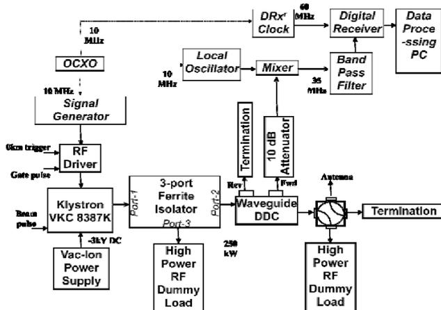
Figure-2 Integrated measurement setup
