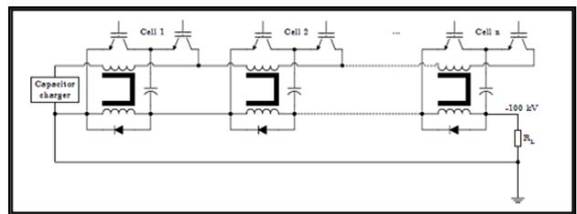
Figure-1 Solid state modulator topology
