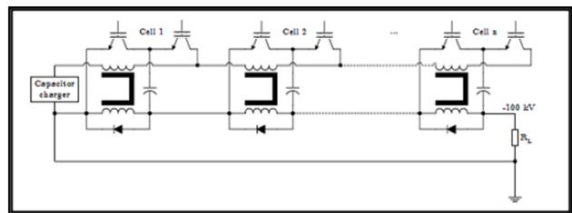
Figure-1 Solid state modulator topology
