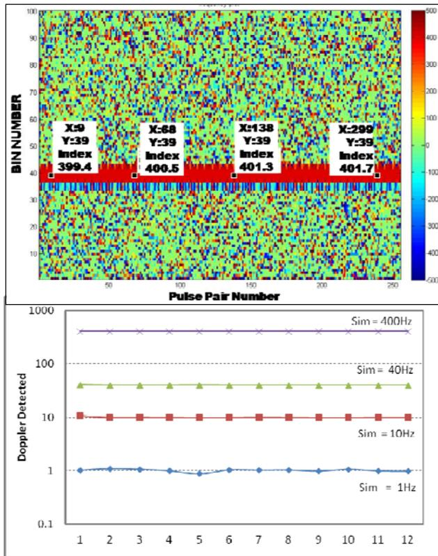
Figure 5(a) Simulated Doppler of 400 Hz detected 5(b) Doppler detection for various values, with averaged value for sets of 20 PRTs for 6 acquisitions
