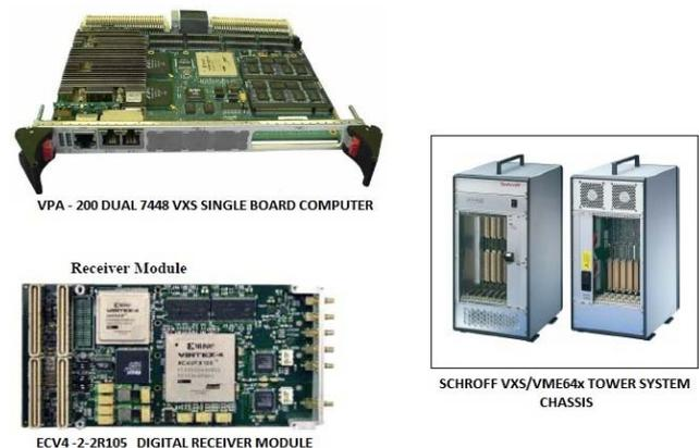
Figure-3 Digital Receiver Hardware
