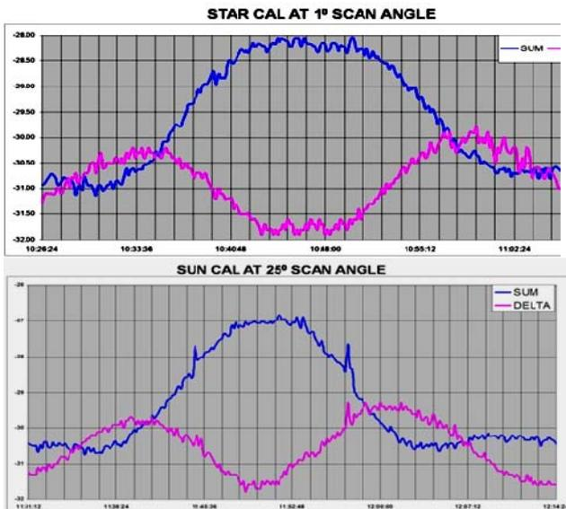
Figure-5 Patterns recorded with Virgo A at 1 deg scan angle and Sun at 25 deg scan angle.
