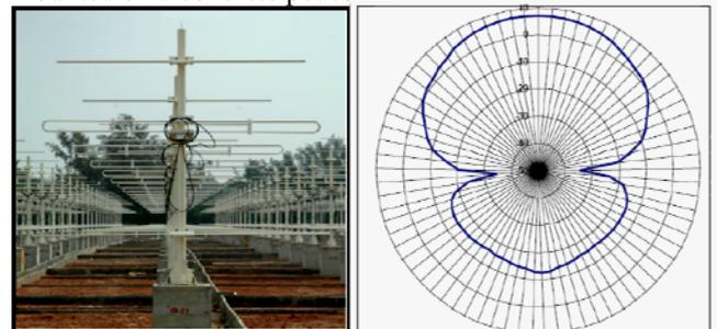
Figure-2(a) Yagi with Folded Dipole,
