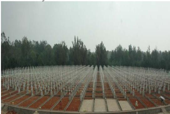
Figure-1 Wind Profiler Antenna Array
