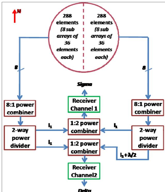
Figure-3 Configuration of the array for the measurement
