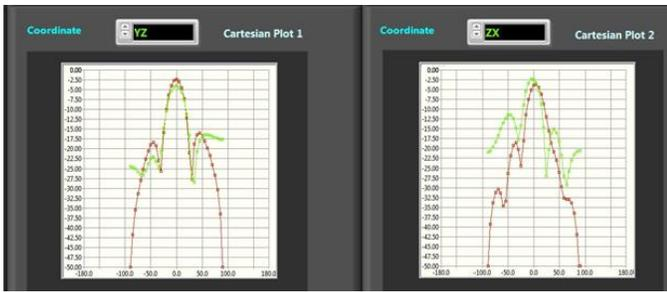
Figure 12: Measured principal-plane radiation patterns of a 4-tile dual-band AESA aperture at 4.8GHz. Left: YZ plane, Right: ZX plane.
