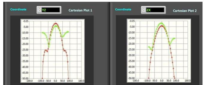
Figure 11: Measured principal-plane radiation patterns of a single dual-band AESA tile at 4.8GHz. Left: YZ plane, Right: ZX plane.
