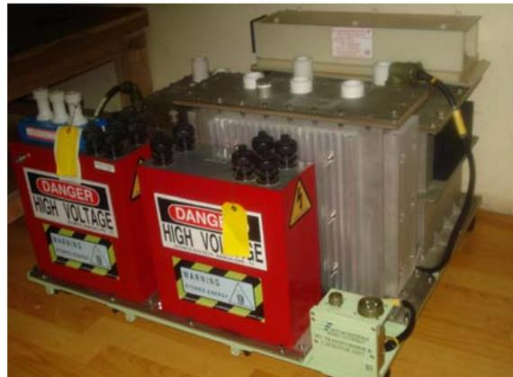
Capacitor & Transformer assembly
