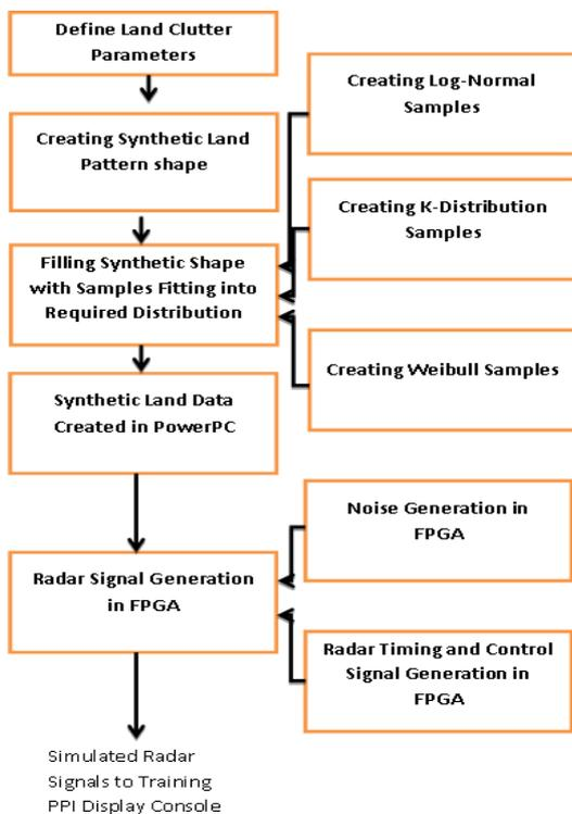
Figure 4: Simulator Algorithm and Signal Flow Chart
