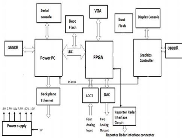
Figure 3: Simulator Hardware Architecture
