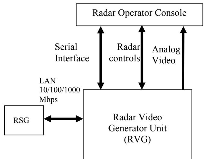
**Figure 1:** Radar Simulator System
