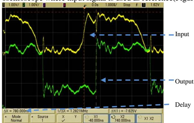
Figure 3 Delay measurement with digital signal
