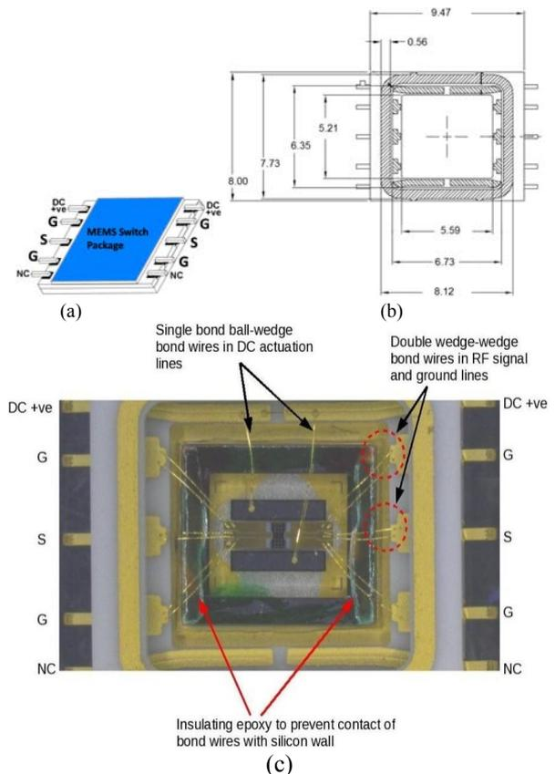
Fig. 3 Surface mount package for the RF-MEMS switch (a) 10 pin package with lid (b) typical dimensions and (c) Packaged RF-MEMS switch with bond wires [7].
