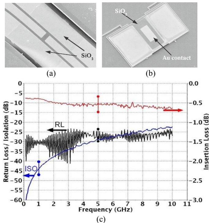
Fig. 2. SEM images of a typical fabricated device [1] (a) CPW lines with the gap in the signal lines (b) Actuator structure (flipped over) (c) Measured S-parameters at die-level.
