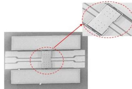
Fig. 1 Top view of the present RF MEMS switch based on Silicon-on-Glass in Co-Planar Waveguide medium with the actuator structure.
