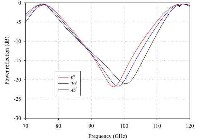
Figure 4 Power reflection characteristics of two-layer metamaterial-FSS for TE polarization at different angle of incidence ( $0^\circ$ ,  $30^\circ$ ,  $45^\circ$ ).
