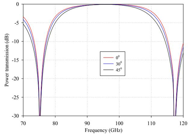
Figure 5 Power transmission characteristics of two-layer metamaterial-FSS for TM polarization at different angle of incidence ( $0^\circ$ ,  $30^\circ$ ,  $45^\circ$ ).
