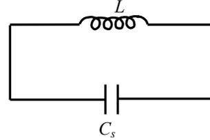
Figure 2 Lumped equivalent circuit of square SRR.
