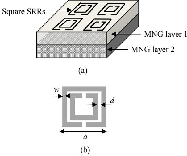
Figure 1 (a) Schematic of a two-layer metamaterial FSS structure, and (b) Geometry of unit cell of MNG layer.
