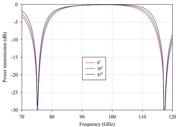
Figure 3 Power transmission characteristics of two-layer metamaterial-FSS for TE polarization at different angle of incidence ( $0^\circ$ ,  $30^\circ$ ,  $45^\circ$ ).
