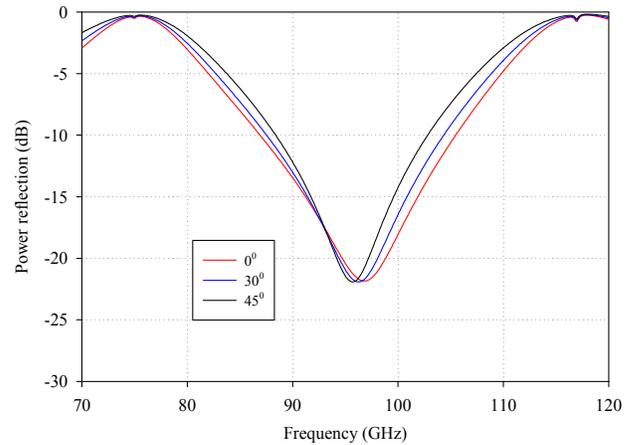
Figure 6 Power reflection characteristics of two-layer metamaterial-FSS for TM polarization at different angle of incidence ( $0^\circ$ ,  $30^\circ$ ,  $45^\circ$ ).
