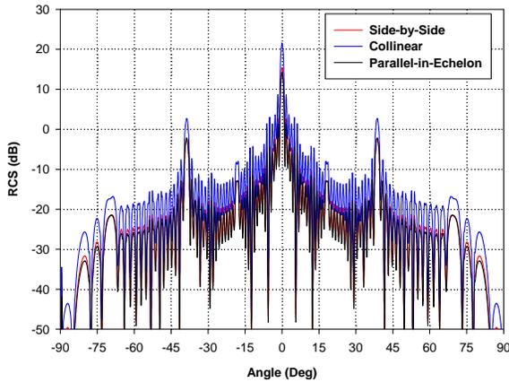
Fig. 3. Effect of array configuration on the RCS pattern of 64-element linear parallel-fed dipole array.
