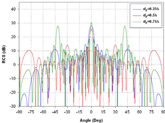
Fig. 5. Effect of inter-element spacing on RCS of 16x10 planar side-by-side dipole array.
