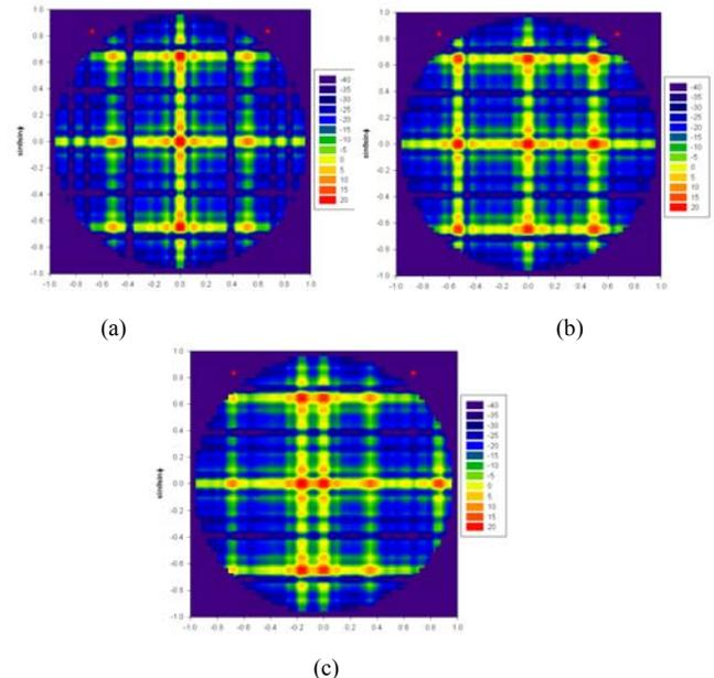
Fig. 6. Effect of beam scanning on RCS pattern of 16x10 planar parallel-fed dipole array (a)  $\theta_s = 0^\circ$  (b)  $\theta_s = 45^\circ$  (c)  $\theta_s = 60^\circ$  RCS pattern of 16x10
