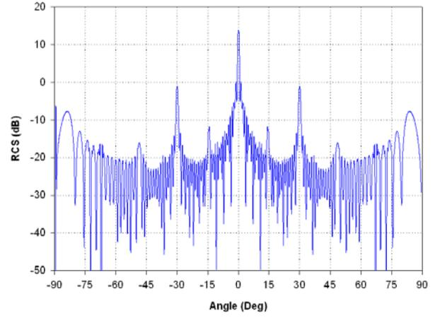
Fig. 1. Broadside RCS of 64-element linear parallel-in-echelon dipole array.
