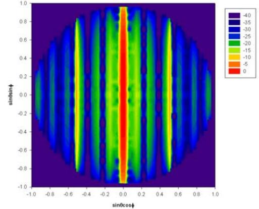
Fig. 2. Contour plot of 64 element parallel-fed linear side-by-side dipole array
