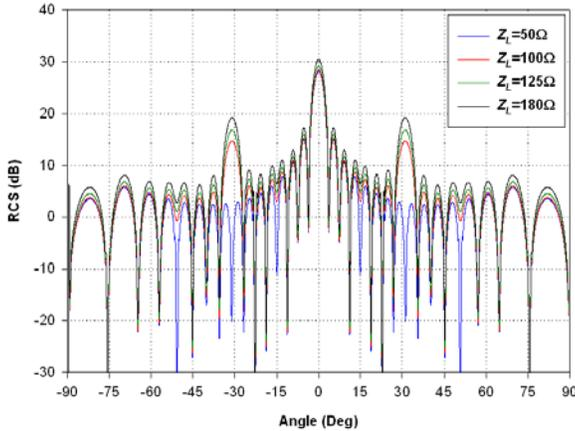
Fig. 4. Effect of terminating load impedance on RCS pattern of 16x16 planar side-by-side dipole array.
