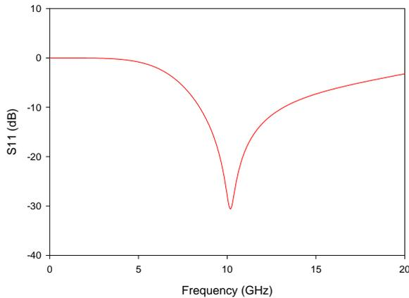
Fig. 4. Return loss characteristic of conformal RAS.
