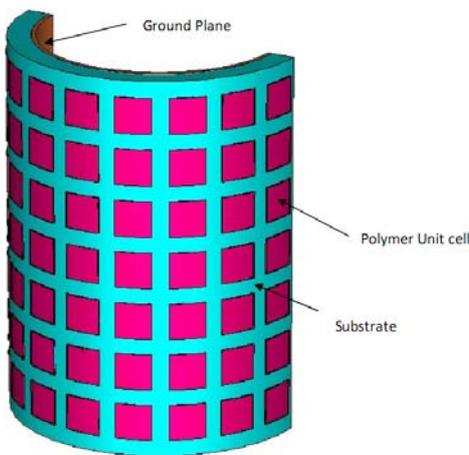
Fig. 2. Schematic diagram of conformal RAS.
