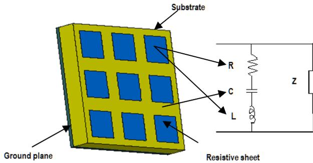
Fig. 1. Circuit analog absorber and Equivalent circuit
