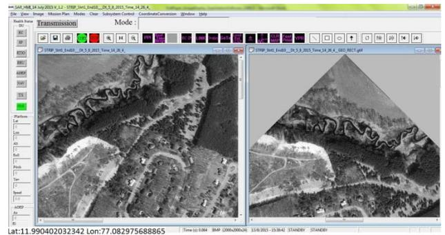
Figure 6 Normal Image and corresponding Georectified & Geocoded Image
