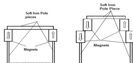
Fig. 2 (a) Focusing structure-I and 2(b) Focusing structure-II
