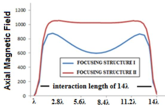
Fig 3 Axial magnetic field for focusing structure I & II
