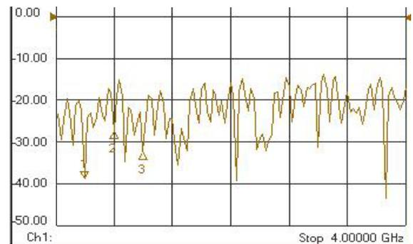
Figure 6. Measured return loss of S-band antenna.
