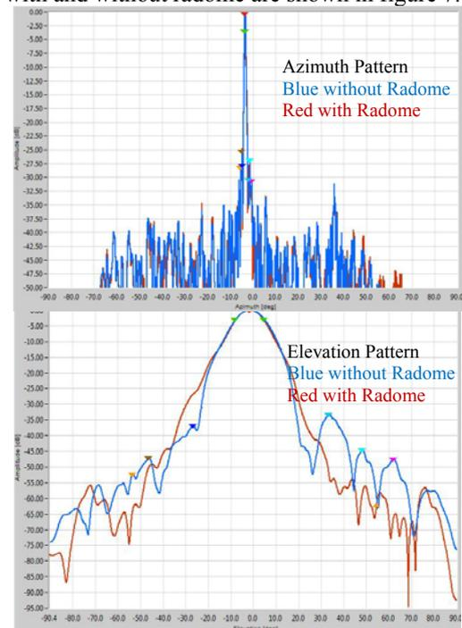
Figure 7. Measured radiation pattern of X-band antenna.
