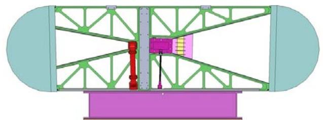
Figure 1. Antenna System for CSR application. It comprises of back to back X-and S-band slotted waveguide travelling wave antenna enclosed in metallic baffles covered with radome.
