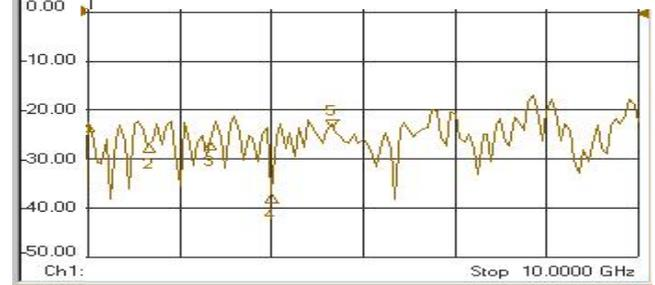
Figure 5. Measured return loss of X-band antenna.
