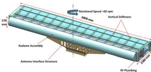
Figure 4. Sub-assemblies / components of CSR Antenna System.
