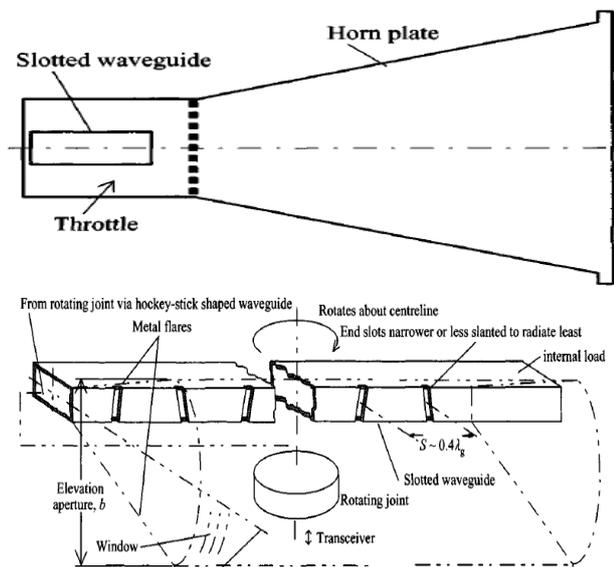
Figure 2. X-band Antenna Configuration for CSR application.
