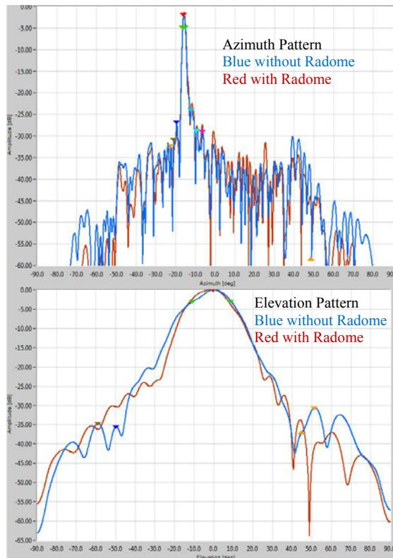
Figure 8. Measured radiation pattern of S-band antenna.
