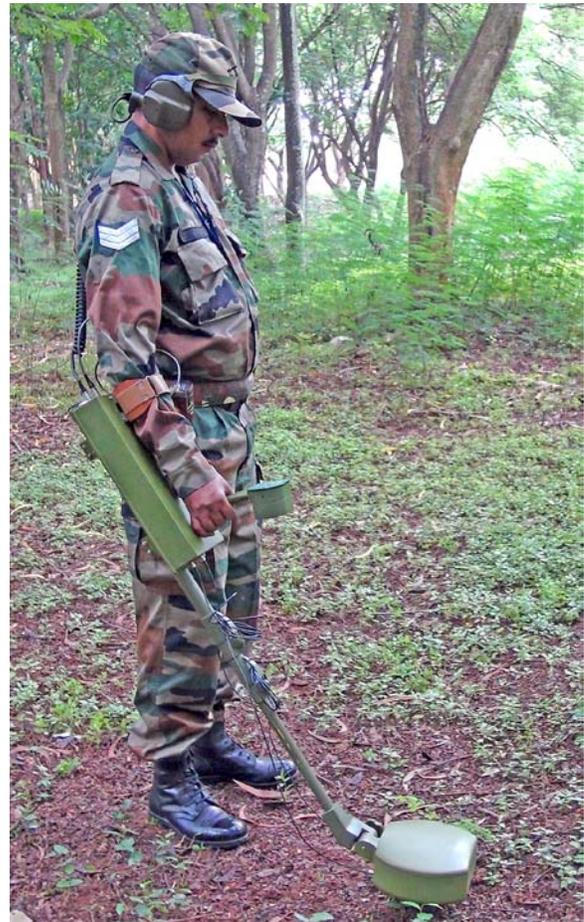
Figure 2: Indigenously realized Handheld GPR
