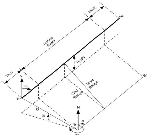
Figure 1 SAR Imaging Geometry
