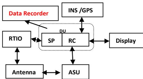
Figure 2 Block diagram of SAR on FTB with data recorder
