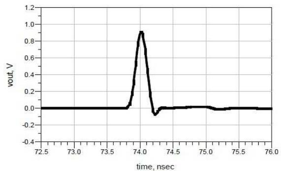
Figure 4 Simulation Result of Gaussian Pulse generator
