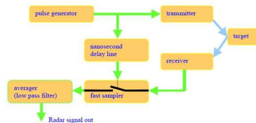
Figure 1 Simplified Block diagram of UWB Radar
