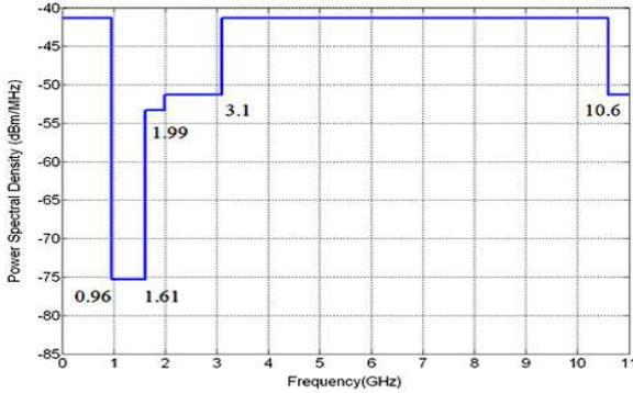
Figure 2 FCC's UWB mask for permissible characteristics
