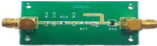
Figure 6 Photograph of Gaussian Pulse Generator Board
