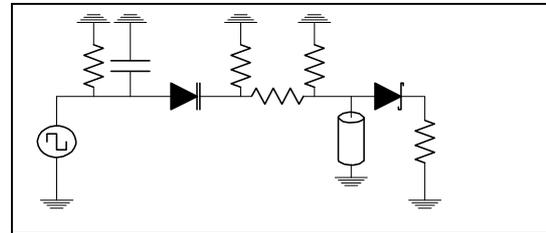
Figure 3 Schematic of Gaussian Pulse generator
