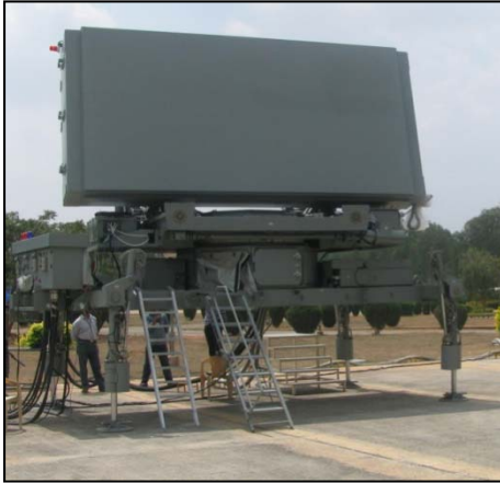
Fig. 8: Realized pedestal assembly with antenna
