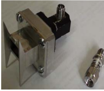
Figure 4. Mechanically Realized Ka-band feed horn.
