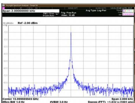
Figure 6. RF output Spectrum with HSR circuit.
