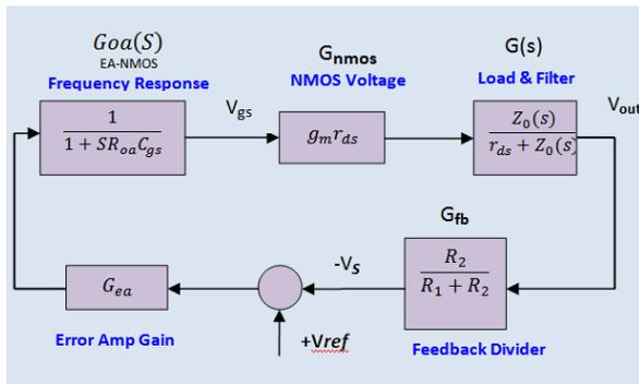
Figure 2. Electrical model of the HSR loop
