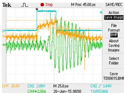
Figure 3. TWT pulsing with 50µSec,30% duty cycle. CH1 Cathode Voltage ,CH2 Grid Pulse TWT, CH4 Inverter current (5.8A peak)
