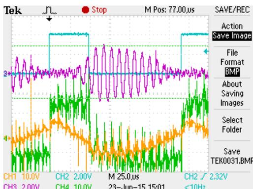
Figure 4. TWT pulsing with 50µSec,30% duty cycle. CH1 Voltage across HSR MoSfet ,CH2 Grid Pulse TWT, CH3 Inverter current (5.8A peak),CH4 Cathode Voltage.
