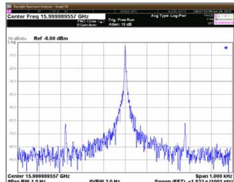
Figure 7. RF output Spectrum without HSR circuit.
