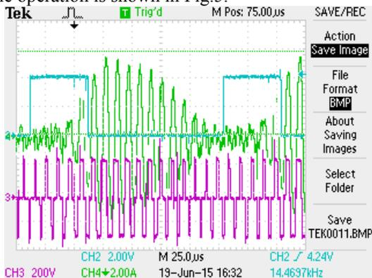
Figure 5. TWT pulsing at 50µSec 30% duty cycle. CH2 Grid Pulse TWT, CH3 O/P voltage of the inverter, CH4 inverter current (5.8A peak)
