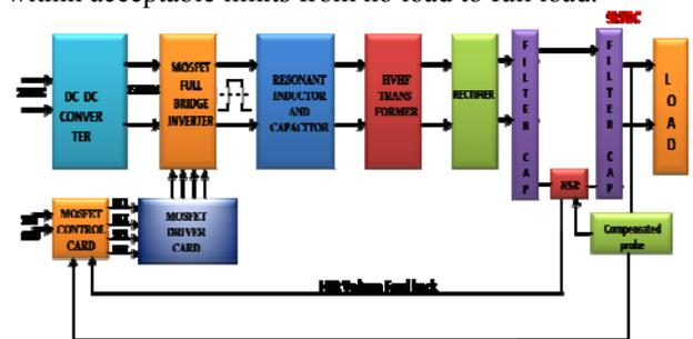
Figure 1. Block Diagram of the TWT Power Supply
