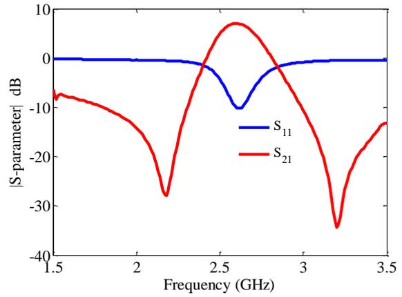
Figure 10. Measured  $S$ -parameters.
