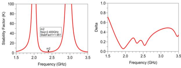
Figure 6.  $K$ - $\Delta$  test based on simulated  $S$ -parameters.
