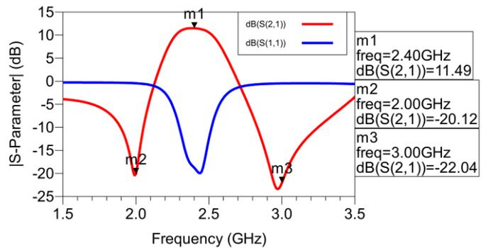
Figure 5. Simulated S-parameters of integrated LNA.
