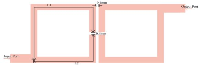
Figure 2. Filter structure.
