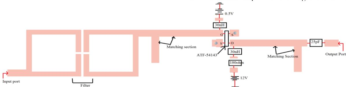
Figure 4. Circuit of the integrated LNA
