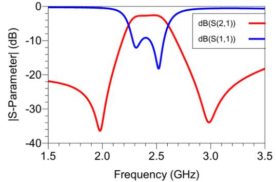
Figure 3. Simulated S-parameters of the designed filter.
