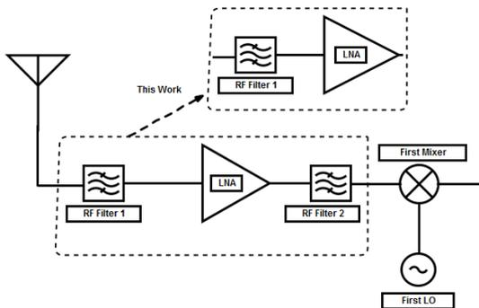
Figure 1. A typical superheterodyne receiver and the present work.
