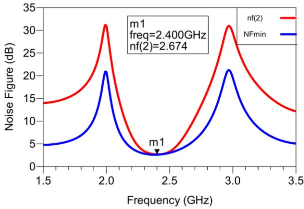
Figure 7. Simulated noise figure of the integrated LNA.
