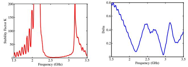
Figure 11.  $K$ - $\Delta$  test based on measured  $S$ -parameters.
