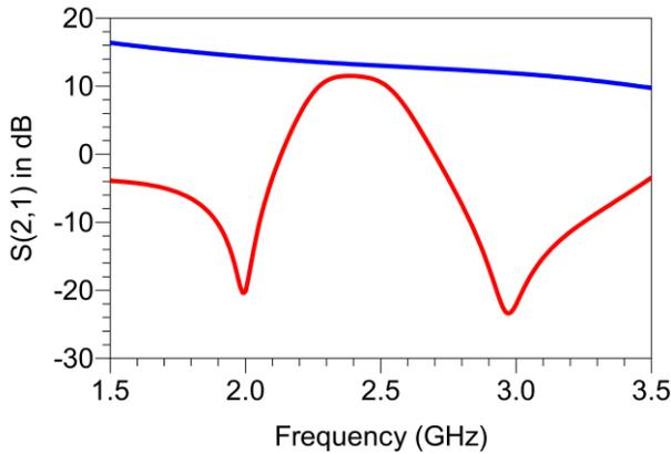
Figure 8. Simulated transmission response of the LNA with (red) and without filter (blue).
