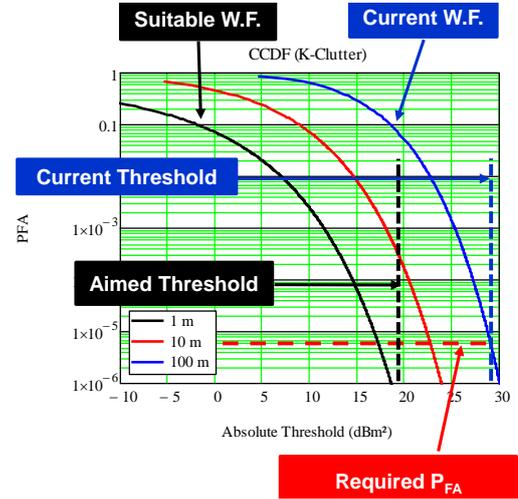
Fig. 6. Method to get a suitable waveform (same  $P_{FA}$  in this example).
