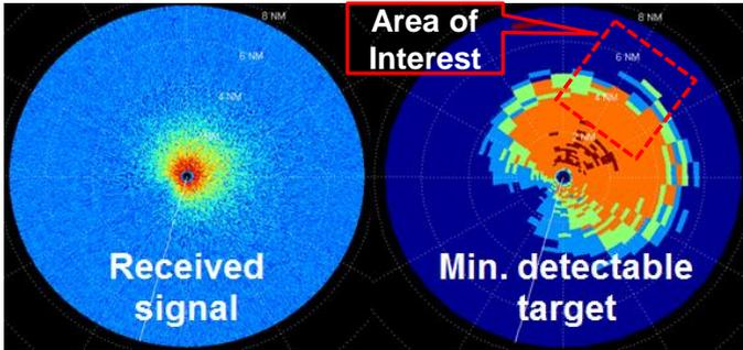
Fig. 2. Raw radar signal (left), map of Minimum Detectable Target (right). The colour indicate the value of MDT: dark blue: very small targets are detectable; orange: only strongest targets are detectable.
