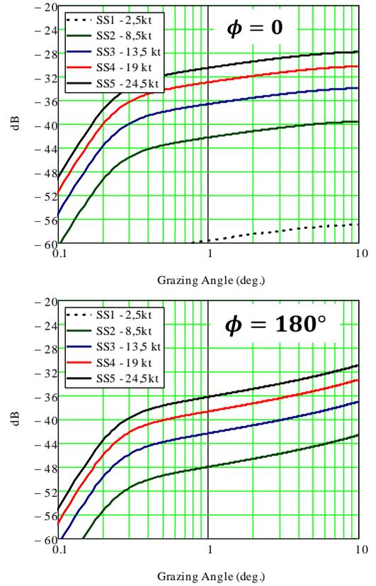
Fig. 4. GIT modelling for two particular aspect angle relative to wind.
