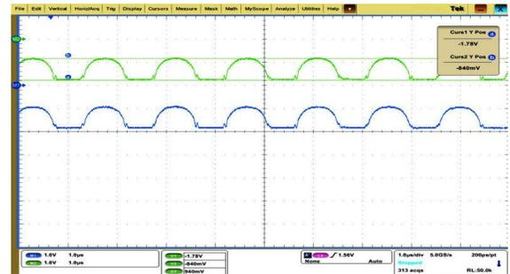
Figure 5. Phase as well gain matched output
