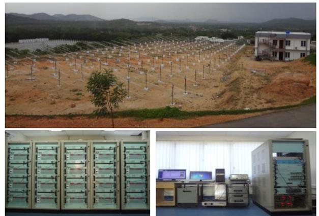
Figure-1: Photographs of the antenna array and the instrumentation building (top panel), transmit-receive system (bottom left) and radar controller (bottom right).
