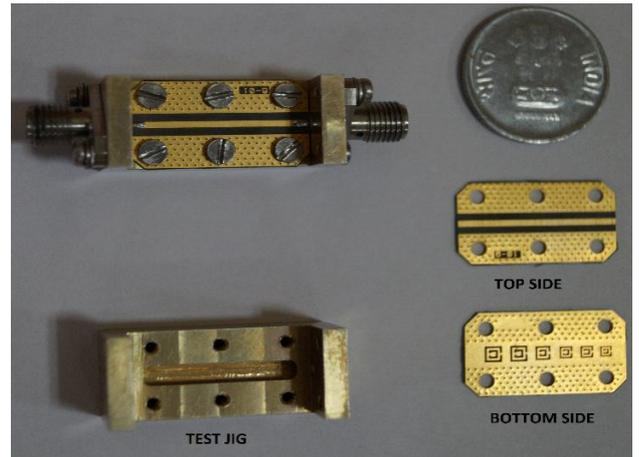
Figure 10 Photograph of DGS-based LPF
