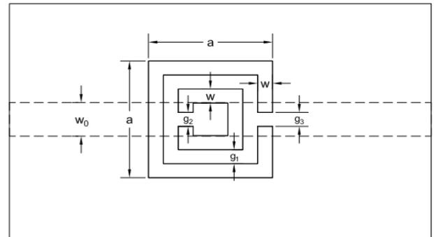
Figure 1 Bottom view of single element DGS with micro-strip line
