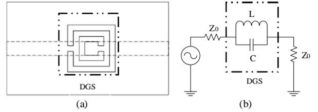
**Figure 5** (a) DGS Single element (b) LC Equivalent circuit
