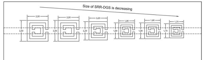
**Figure 6** Cascaded elements of DGS
