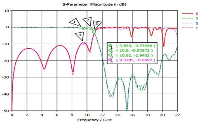
Figure 9 EM Simulation Results for LPF
