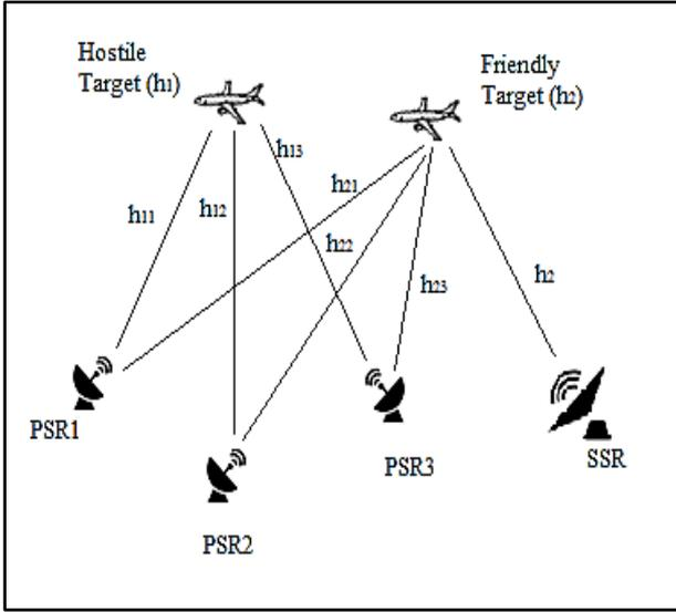
Fig. 1: Problem Statement: Three primary radars (PSR1, PSR2, PSR3) and one SSR
