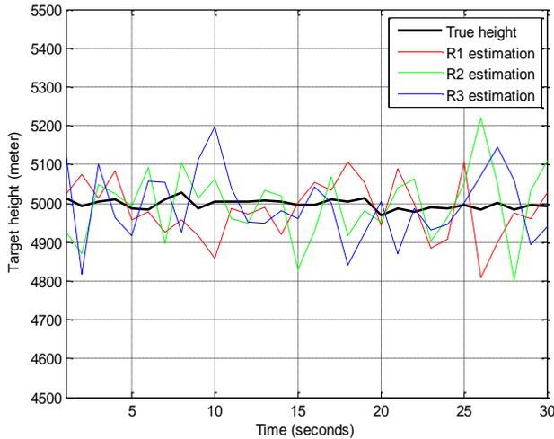
Fig. 3: Target height captured by various PSRs and the true height of the target
