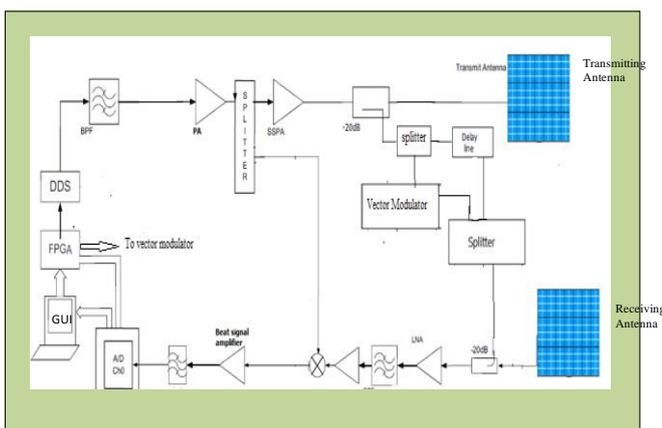
Fig. 3 Block Diagram of FMCW radar – DBS mode
