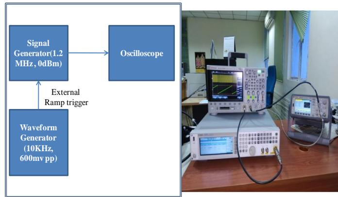
Fig. 5 Waveform synthesis test setup
