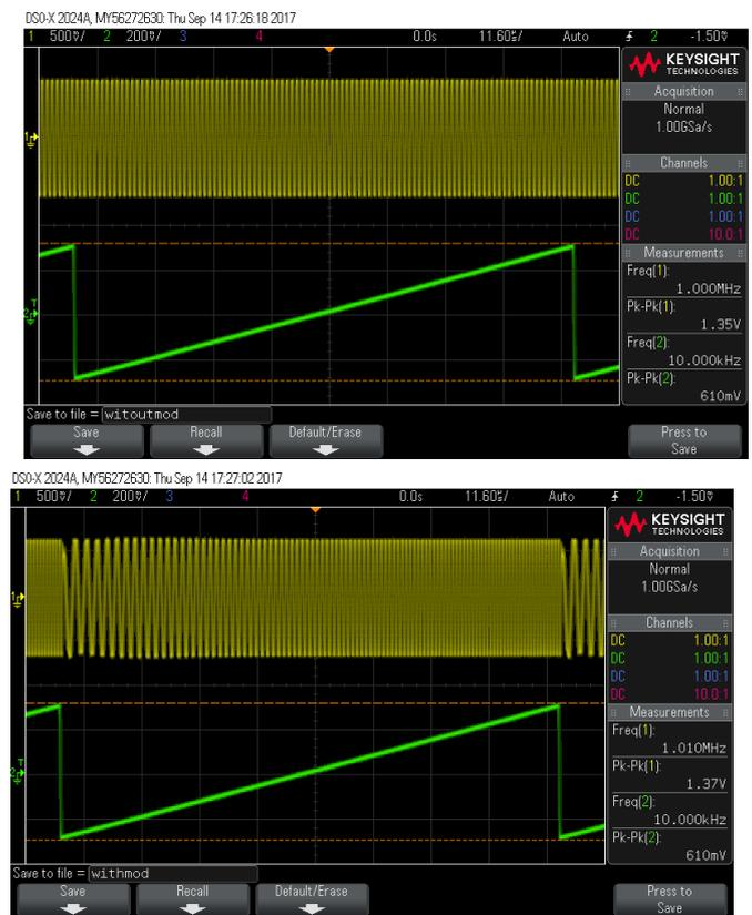
Fig.6 Synthesized Waveforms of CW signal without (top) and with (bottom) FM modulation
