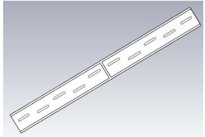
Fig. 2 Top view of 1x10 linear slotted waveguide array.
