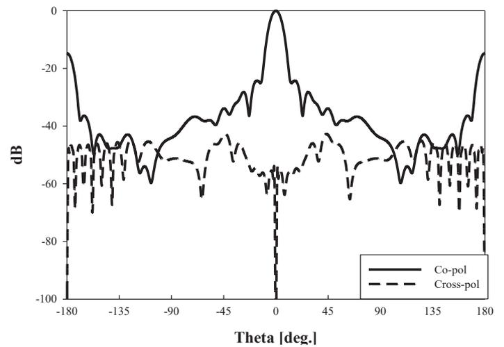
Fig. 6. Radiation pattern of 10 element array.
