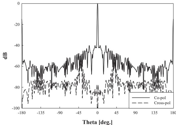
Fig. 7. Radiation pattern of 150 element linear array.
