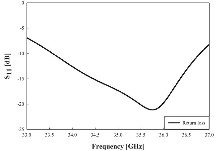
Fig. 5 Return loss characteristic of slotted waveguide array.
