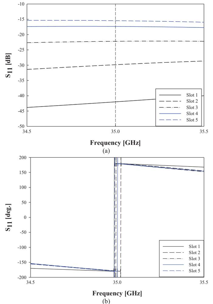
Fig. 3. Return loss of individual slot radiators (a) Magnitude in dB (b) phase in degree.
