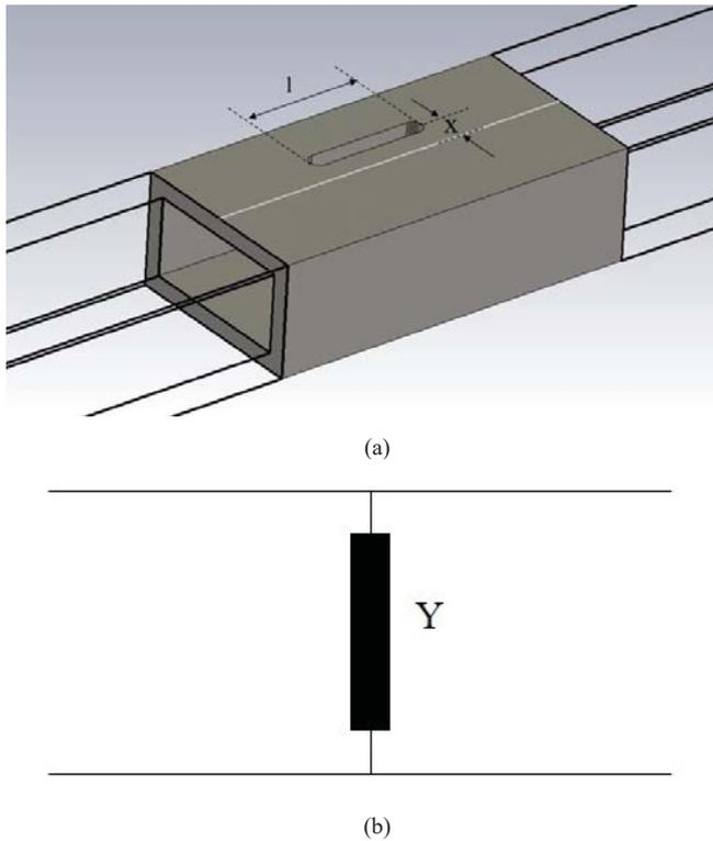
Fig. 1 Single slot radiator (a) Simulated model (b) Equivalent circuit.
