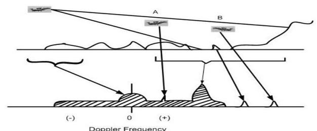
Fig. 1. Clutter spectrum for an airborne radar
