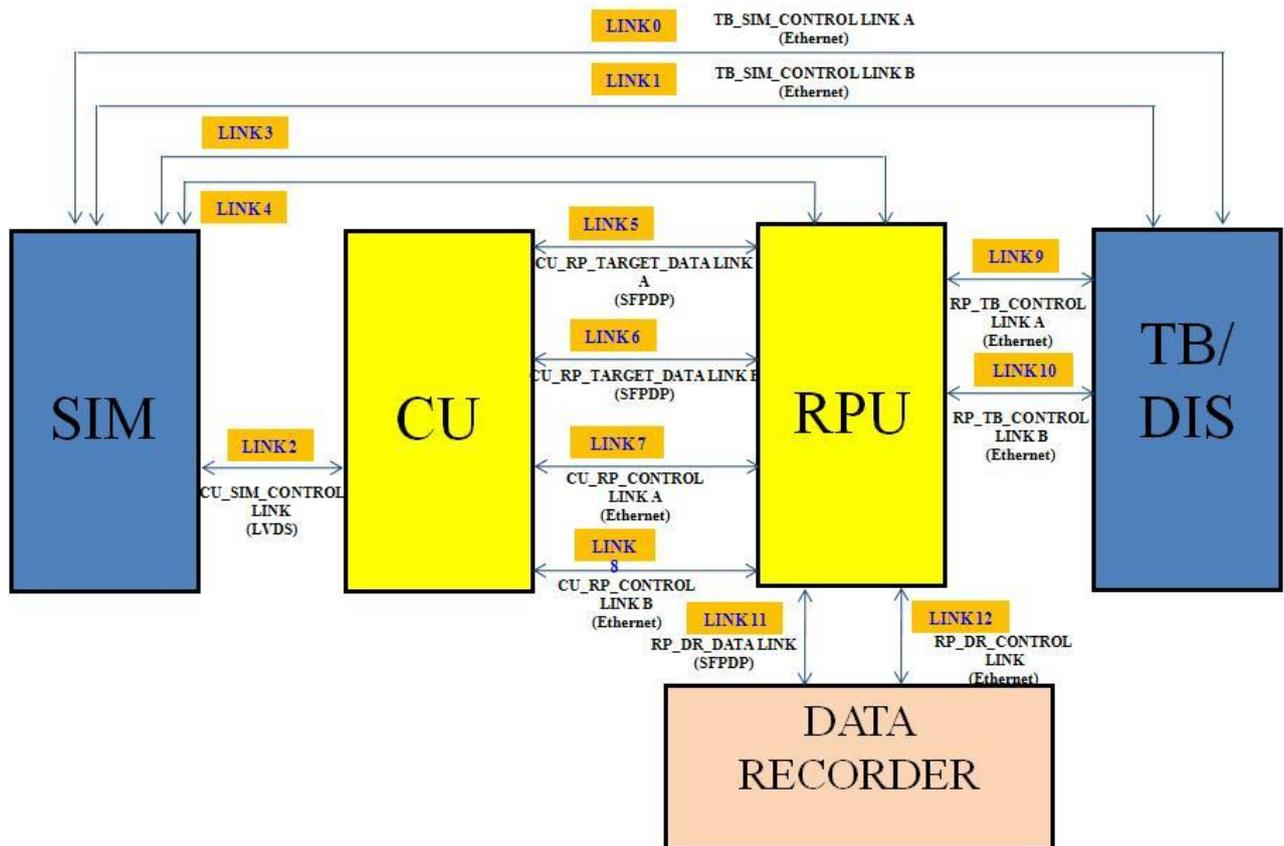
Fig. 5. An Interface Diagram of Digital Environment Simulator
