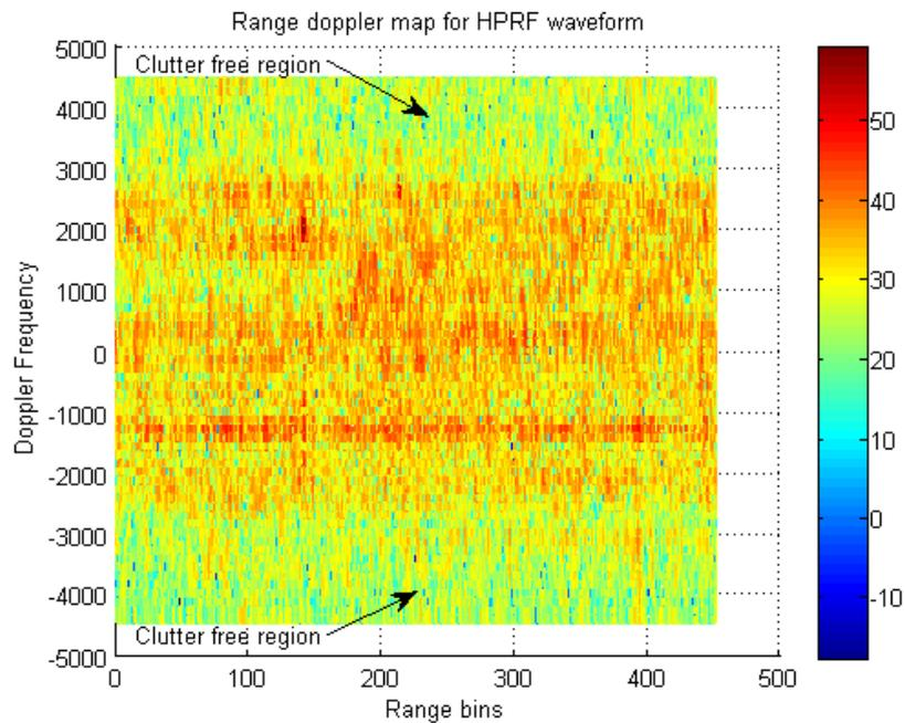
Fig. 7. The Range Doppler map. The bright stripes are ground clutter seen through the sidelobes of the antenna
