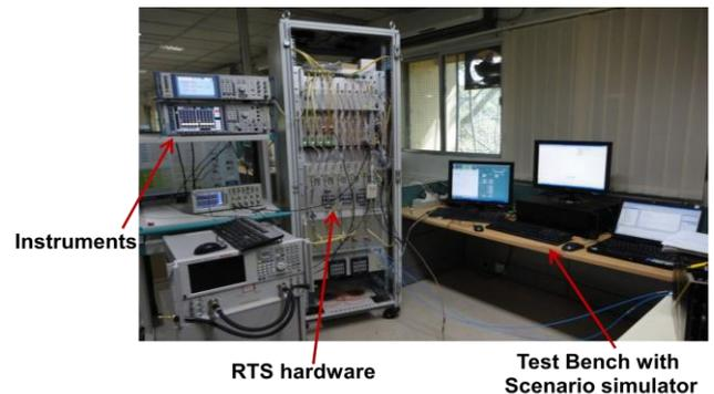
Fig. 3. Major elements of Radar Target Simulator
