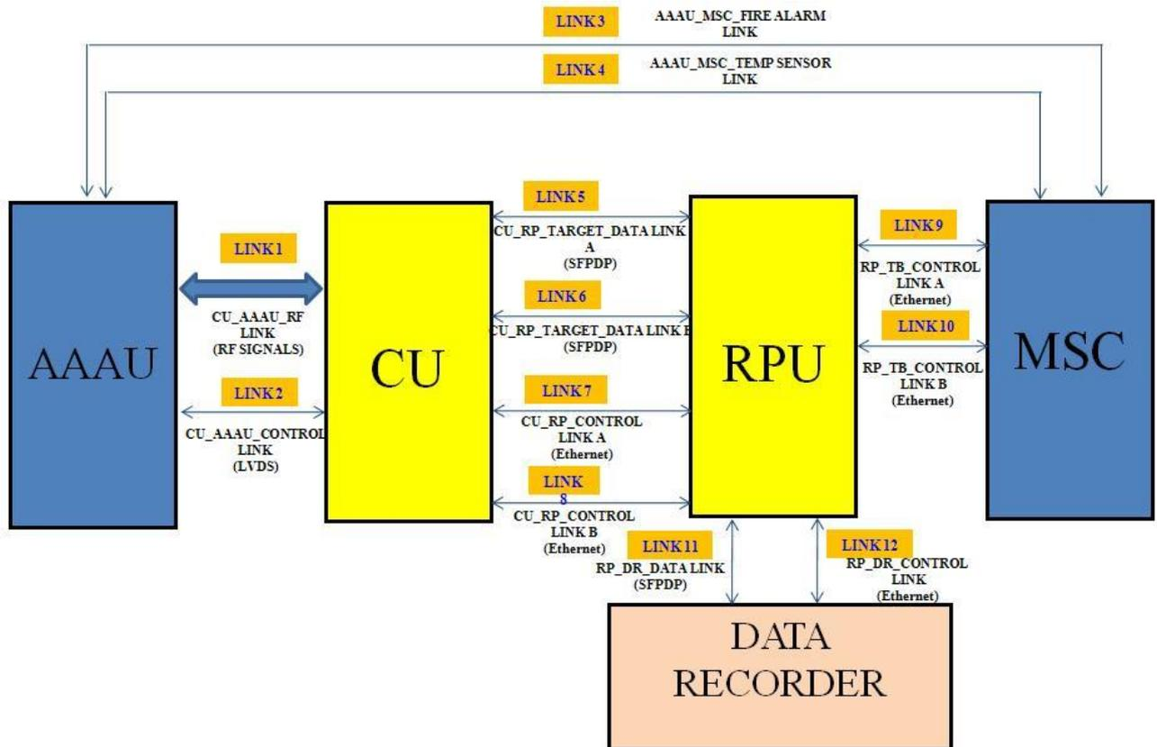
Fig. 6. An interface diagram of the principal test bed computer systems. MSC coordinates, and represents the primary operator interface for controlling the test bed systems.
