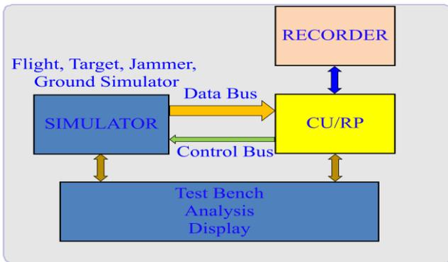
Fig. 4. Block Diagram of Digital Environment Simulator
