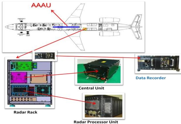
Fig. 2. Principal elements of the Airborne Radar Test Bed
