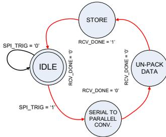
Figure 4: SPI Slave Module State Machine
