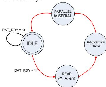
Figure 6: SPI Master Module State Machine
