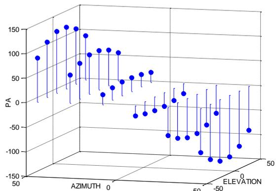
Figure 8: Phase Gradient (P<sub>A</sub>) Plot with Azimuth and Elevation Angles
