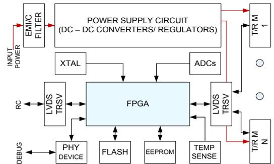
Figure 3: PGC Hardware Architecture
