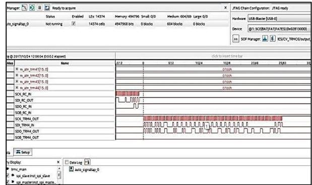
Figure 11: Data Interface between PGC and T/R Module
