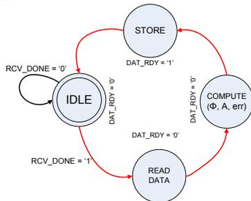
Figure 5: Computation Process Module State Machine
