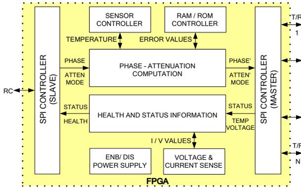
Figure 2: Functional Block Diagram of PGC
