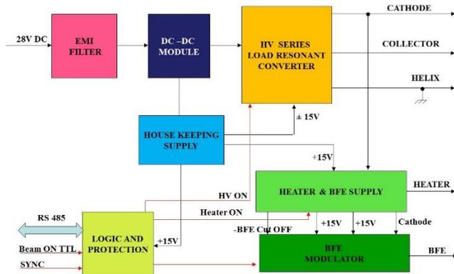
Figure 2 Block diagram of EPC
