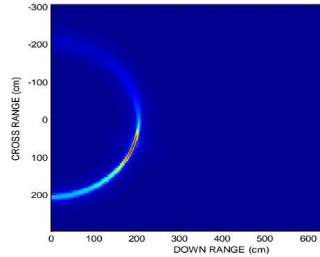
Figure 6(b) Image obtained using 8192 point IFFT and time domain backprojection
