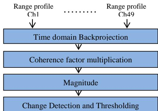
Figure 2 2D Imaging scheme
