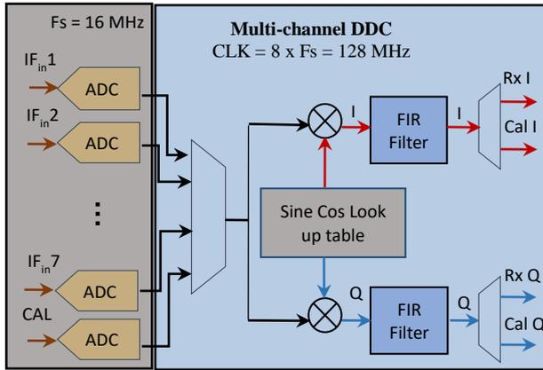
Figure 3 Multichannel Digital down conversion
