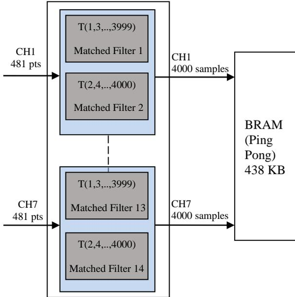
Figure 8 Multiple instantiation of matched filter
