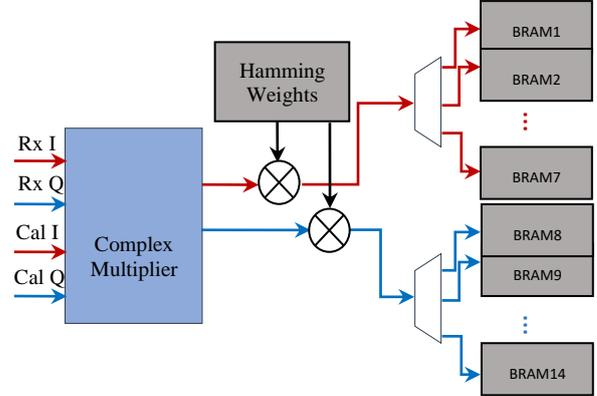
Figure 4 Calibration and windowing
