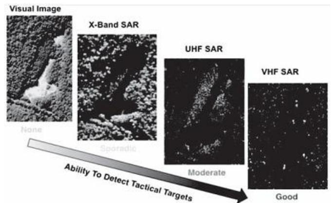
Fig 1: Comparison of optical image and RADAR image sources [1]
