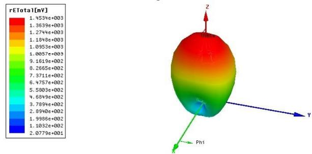
Figure 4: Electric field intensity pattern at 130 MHz
