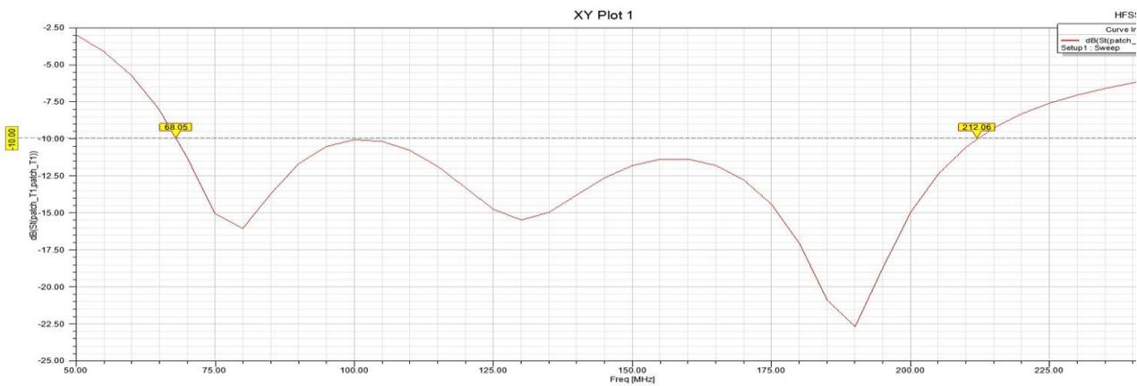
Figure 3: Return loss(dB) Vs Frequency(MHz)
