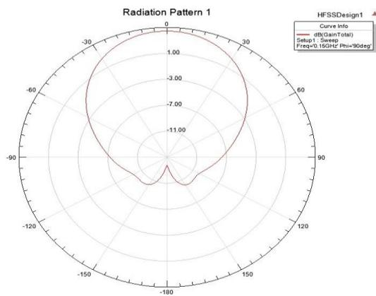
Figure 5: Gain pattern at 150MHz
