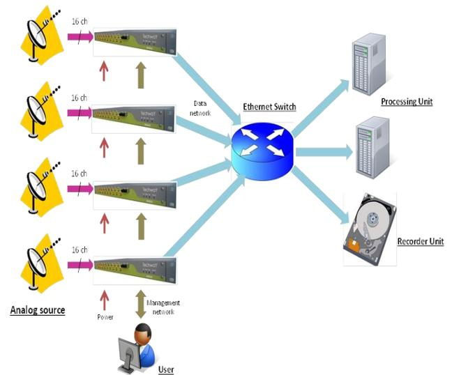
A new concept developed based on fully independent and versatile data-acquisition front-end with embedded FPGA processing capabilities. Front-end can be an industrial PC , with latest FPGA PCI Express form factor card, programmable at a higher level rather than HDL.
