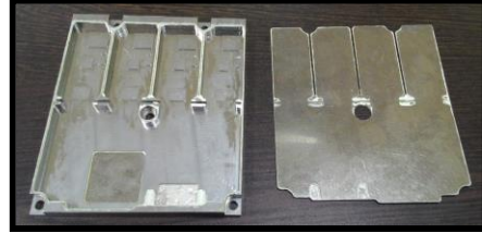
Figure 3: Mechanical Housing of QTRM Top cover lid opens after HALT Vibration step stress Test
